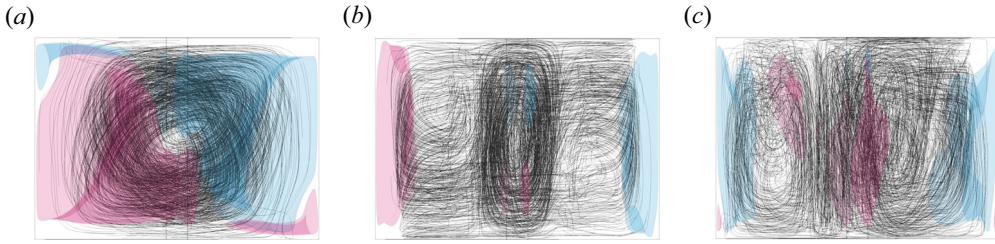
Figure 9. Mean vertical velocity isosurfaces u_z = \pm 0.1 (a) and u_z = \pm 0.05 (b,c) (pink/blue), and streamlines of mean flow (black), from the angled side view. (a) Ha = 200 , Ra = 10^7 ; (b) Ha = 1000 , Ra = 2 \times 10^7 ; (c) Ha = 1000 , Ra = 5 \times 10^7 .
