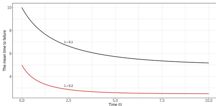
Figure 8. The mean time to failure in Example 4.6 for values  $\lambda = 0.1$  and  $\lambda = 0.2$ .
