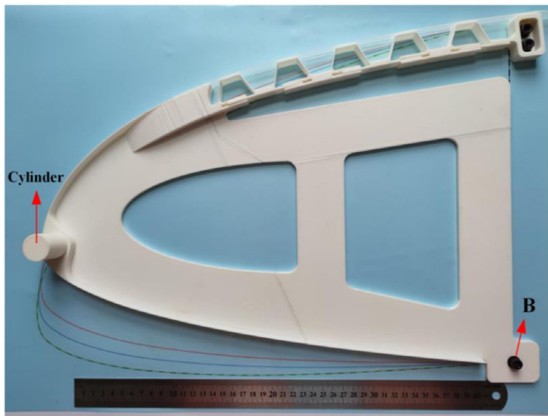
Figure 23. Demonstrator of drooping leading edge with the ICFS.
