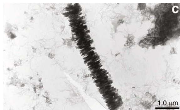
Figure 2. TEM images of complex crystals in which \text{Al}(\text{OH})_3 polymorphs have co-crystallized at pH 12.0 and at a tartaric acid/Al molar ratio of 0.1, showing (a and b at higher magnification) long stick-shaped crystals formed by elongated core units (gibbsite) covered by aggregates of thin platy particles of nordstrandite and (c) long crystals without the 'stick core'.
