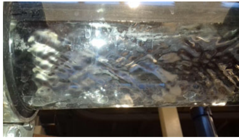
FIGURE 5. (Colour online) Photo of example standing wave at pipe exit when flow is in super-critical regime.
