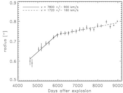
**Figure 4.** ACIS expansion measurements of SN 1987A.
