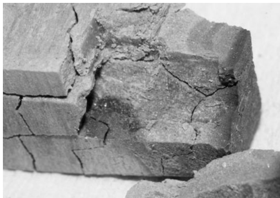
Figure 2. Calcigel clay (ABM1). The dark area to the right is 1 cm \times 1 cm in size and was in contact with the heater. The cracking was caused by the low humidity in the argon glove box.
