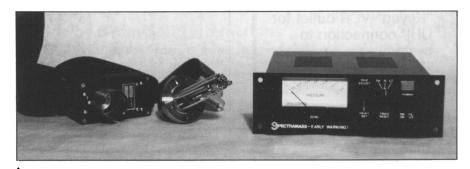
Hydrogen/Helium Leak Detector: The Early Warning Hydrogen Monitor from Spectramass utilizes quadrupole technology to provide three basic functions on cryopumped systems. The equipment accurately monitors the cryopump's life by monitoring the chamber's hydrogen partial pressure. It can also monitor the total
