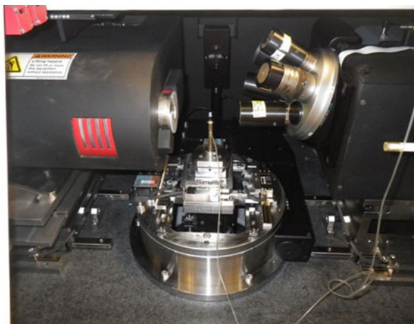
Figure 4. Sample mounted within the X-ray CT system.
