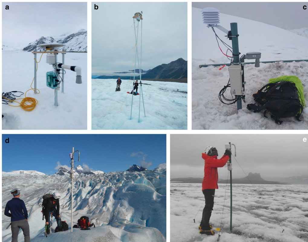
Figure 2. Automated ablation-stake deployments. (a, b) Kennicott Glacier, Alaska, USA: (a) Installation, 17 May 2012; (b) after melt season, 16 September 2013 (possibly a different station). Pictured: (left) Billy Armstrong and (right) Katy Barnhart. (c) Glaciar Hans Meyer, Chimborazo, Ecuador: 29 June 2016. (d) Glaciar Perito Moreno, Argentina: 13 March 2020. Pictured: (left) Max Van Wyk de Vries and (right) Andy Wickert. (e) Glaciar Fourcade, King George Island, Antarctica: 25 January, 2021. Pictured: Matias Romero.
