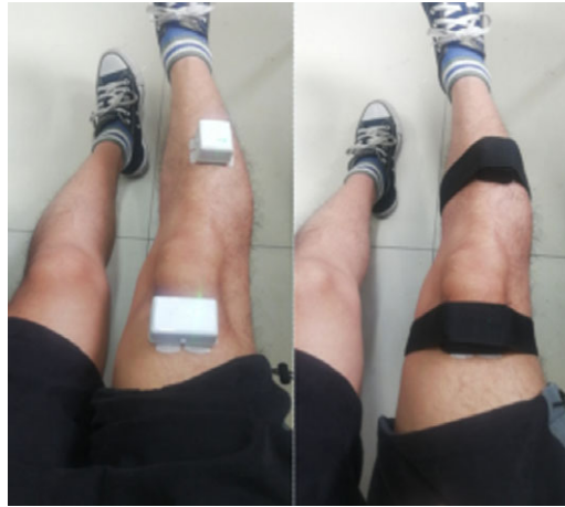
Figure 3. Positions of sEMG acquisition instruments.
