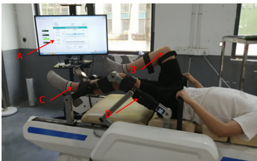
Figure 12. Real-time rehabilitation training in the lying mode (“A” is the upper computer interface, “B” is the healthy side limb of the subject, “C” is the affected limb of the subject (hypothesis), and “D” is the left mechanism of the lower limb rehabilitation robot in the lying training state).
