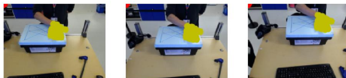
(b) Tracking using Mediapipe on three cameras simultaneously to identify 21 points on the hand and using the (x, y) data to predict the (x, y, z) if the points were the HMD in the virtual world.
