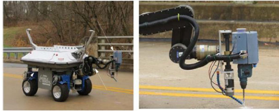
Figure 3. Mobile manipulator-based non-destructive rehabilitation system for bridge deck repair (Gucunski et al., 2015).
