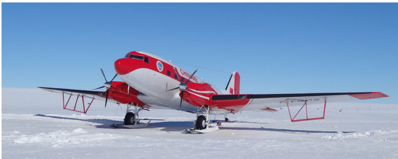
Fig. 1. The Snow Eagle 601 fixed wing ski-equipped aircraft comprising the Chinese polar airborne geophysical platform equipped with RES (the Snow Eagle IPR), gravity, magnetometer, GPS and other instruments.
