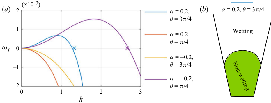
Figure 2. (a) Growth rate, \omega_I , as a function of wavenumber k in the case of equal-density fluids ( R = 1 ). The curves are calculated using the method in § 3. The critical wavenumbers predicted by (4.3) are shown as crosses. We use Bo = 5, h = 0.5, b_0 = 0.3, M = 2, \mathcal{A} = 1 and C = 1 . (b) Schematic corresponding to the blue curve.
