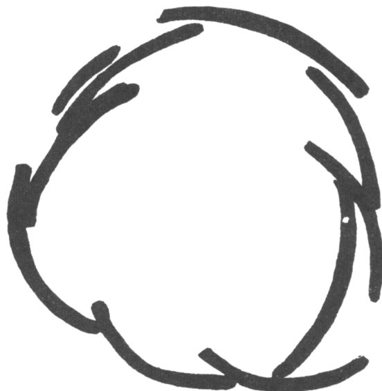
Fig. 11. Model of illite floccule in distilled water. Model is based upon the interpretation of illite fabric in Fig. 10.
