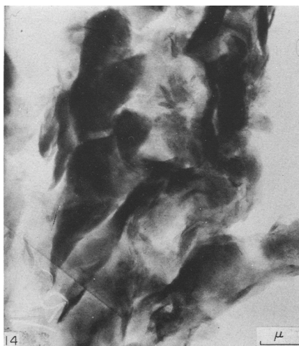
Fig. 14. High voltage electron micrograph of polyethylene glycol impregnated flocculated grundite illite (5 g/l. clay concentration in salt water, 1 g/l. NaCl). Scale 12,800 ×.
