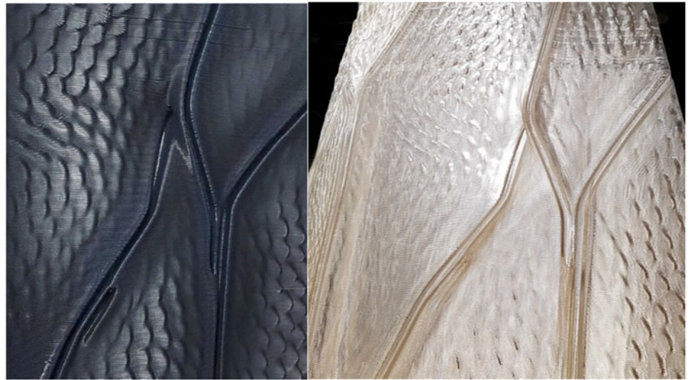
Figure 3. Fibre hemp ropes laced within grooves prefabricated within the scaffold for additional tensile strength.
