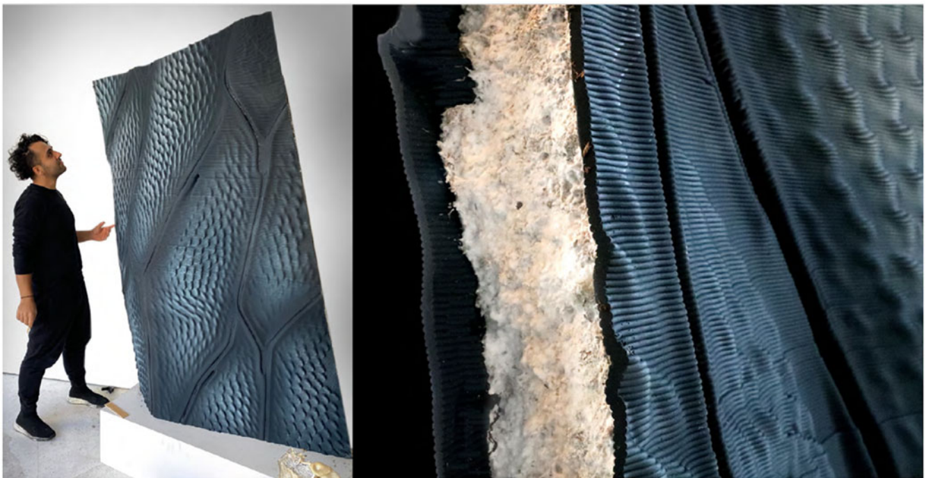
Figure 6. Mycelium growing inside the two-metre high wall panel system.
