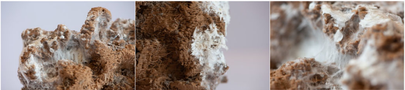
Figure 9. Mycelium growing throughout the 3-D printed wooden skins exposing contrasting biological patterns of growth.
