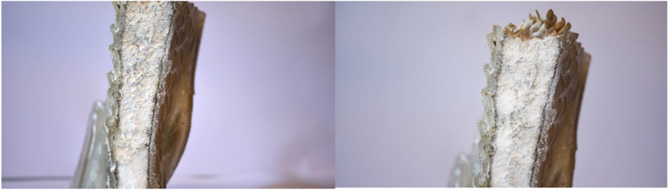
Figure 1. Prototype 01: Mycelium growing inside recycled PETG skins.
