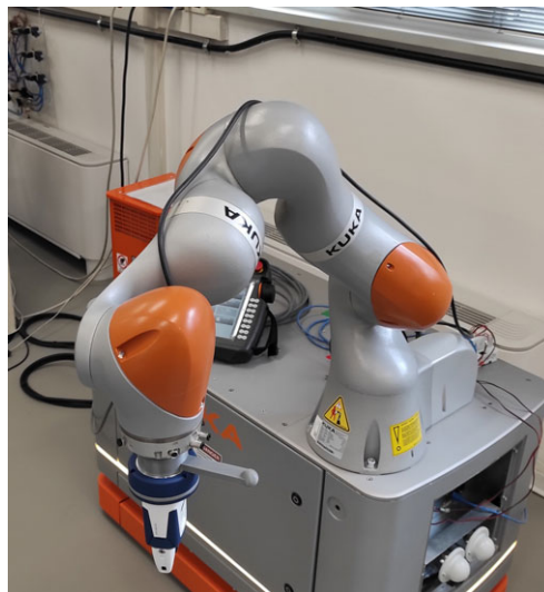
Figure 15. The redundant articulated robot exploited for the experimental validation of the proposed formulation for the kinematic directional index (KDI).
