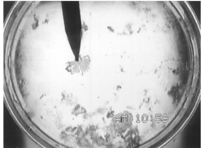
Fig. 5. A typical frazil crystal filmed during experiment D; the diameter of the glass plate is 90 mm.
