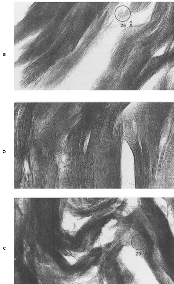
Figure 3. Electron micrograph of the pillared clays prepared from both types of silicon compounds: a and b) different zones of a sample prepared from trichlorosilylethylpyridine; and c) sample prepared from aminopropyltrimethoxysilane.
