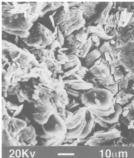
Figure 3. Aggregates of authigenic kaolinite within primary pores of the Utrillas sandstones.
