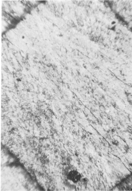
PLATE 1. Rolled test piece, section perpendicular to the plane of preferred particle orientation. Crossed polars, 45^\circ position, maximum illumination ( \times 35 ), (001) N.W.-S.E.
