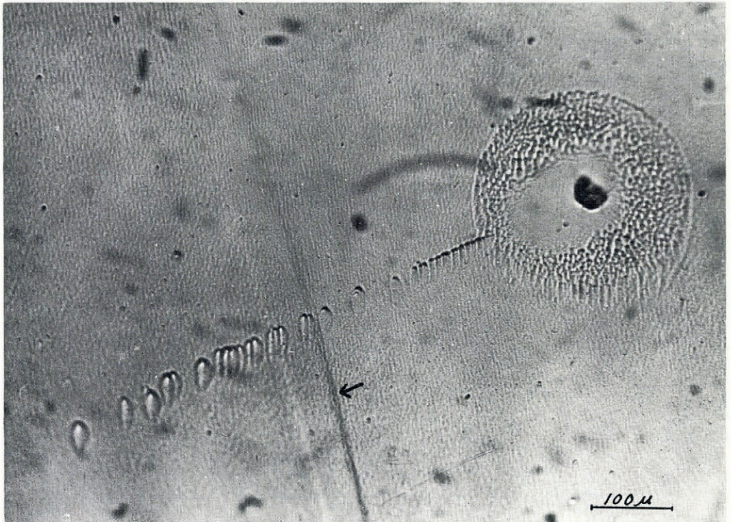
Fig. 5. Sand grain in Mendenhall glacier ice surrounded by cloud of dislocation etch pits. Row of etch pits running diagonally across figure suggests that sand grain acts as source for dislocations. Photograph by Kuroiwa and Hamilton (1963, p. 54). Copyright by M.I.T. Press; reproduced with permission.
