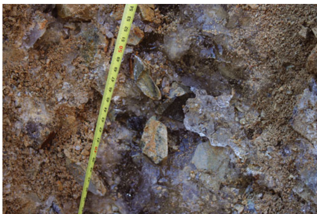
Fig. 6. Coarse-grained, ice-rich (excess ice) and saturated frozen soil found in a test pit at \sim 3 m depth in an active rock glacier in the Andes. (Photo: L. Arenson 2009.)
