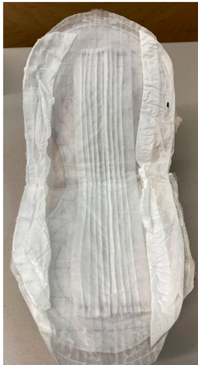
Figure 20. Prototype of integrated diaper pad, later placed into the outer diaper fabric.
