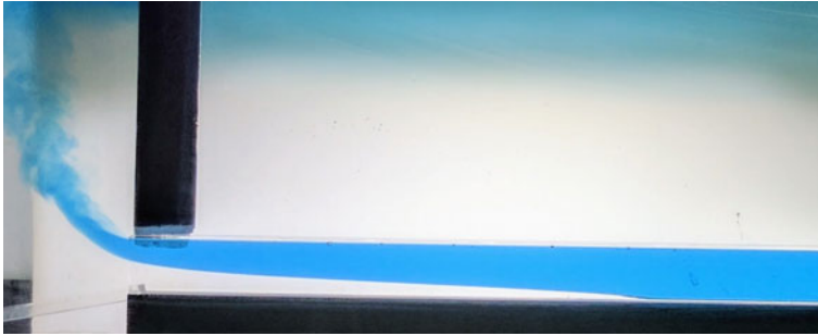
FIGURE 4. A closeup image of an intruding salt wedge during an experiment. Here, freshwater (dyed blue) is observed exiting the channel as a salt wedge intrudes the lower portion of the channel. The freshwater plume and the diluted mixed layer are visible in the left and upper sections of the image respectively.
