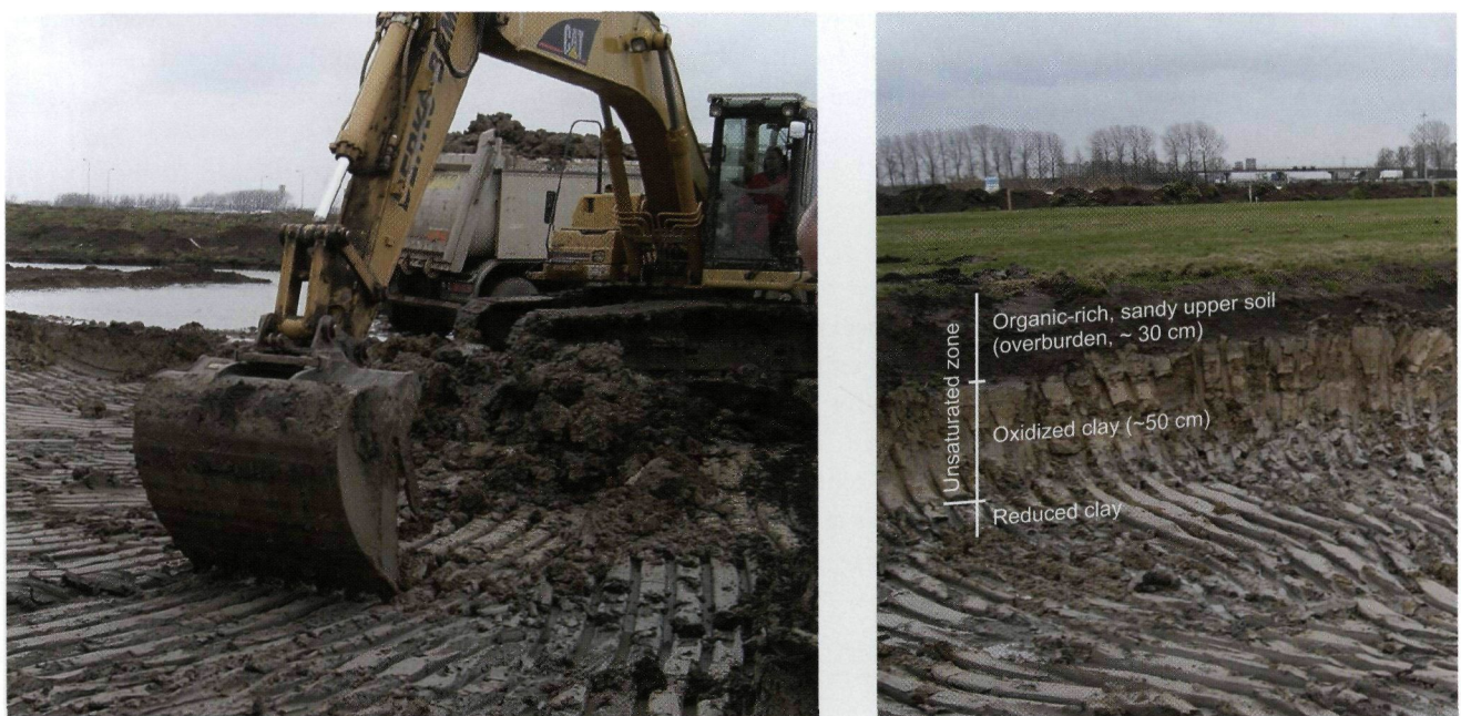
Fig. 6. Left panel: the extraction of clay using a backhoe, near the town of Arnhem (Fig. 2). Right panel: the extraction depth is about 1 m (including ~30 cm of overburden); relevant lithological variation on that vertical scale is clearly visible. A caliche-horizon within the oxidised clays (not visible on this scale) presents a challenge, as it has to be removed before continuing extraction. Photo: DM.
