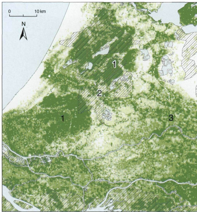
Fig. 10. Detail of the clay-resource maps of the Netherlands (see Fig. 9 for location and legend), showing a number of adequately reproduced geological features: 1. clay surfacing as a result of extraction of the overlying peat in mediaeval times; 2. the tract of a former Rhine distributary; 3. channel-belt architecture below the Rhine-Meuse river plain.
