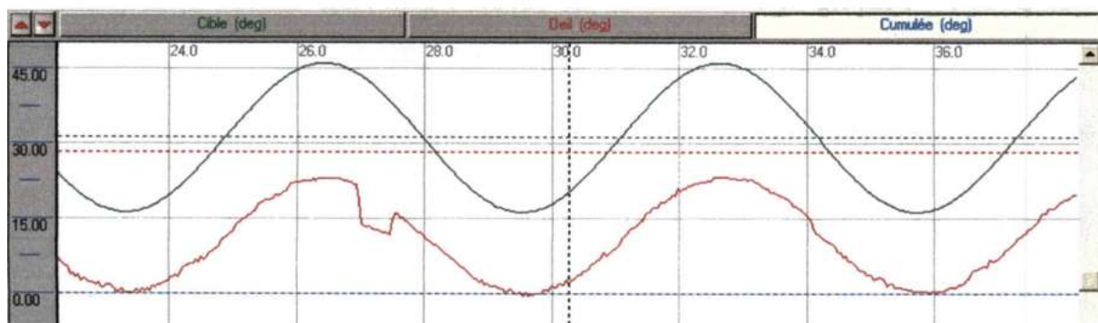
B : Visualization of flutter during vertical ocular pursuit test (green/top = target, red/bottom = patient eye)
