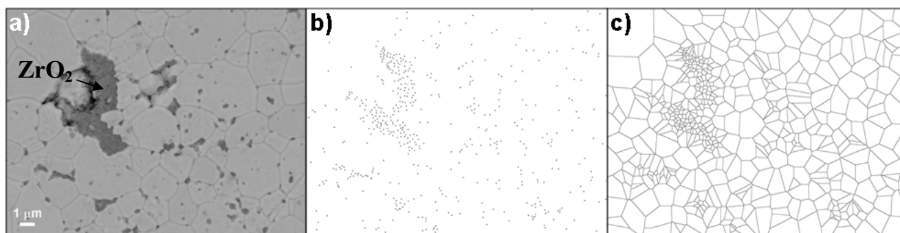
Figure 1. SEM-BE micrograph of the PZT-TZ, after sintering at 1275 °C, 2h (a), points representing the zirconia grains (b) and the Voronoi diagram representing the zirconia distribution (c).
