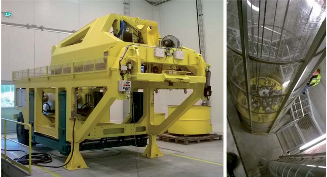
FIG. 5. Left image: the buffer installation machine in the test hall during the lifting test. Testing is done with a concrete block. Right image: the vertical deposition hole, a concrete test block is being lowered to the bottom.
