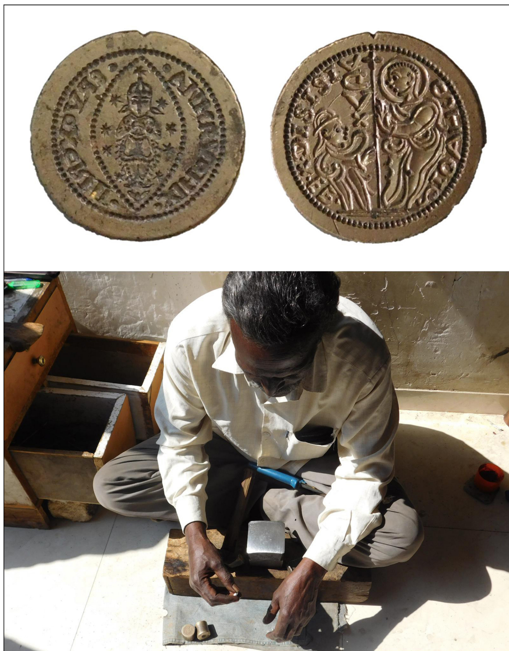
Figure 4. Top) hand-made dies; bottom) the striking of putali (photographs by E. Smagur).
