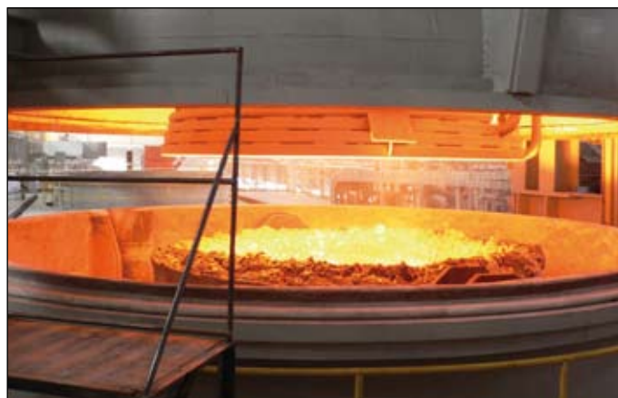
Water-cooled, copper-plated ladle inner roof enables the distance between the melt and the edge of the vessel to be reduced to about 500 millimeters.
