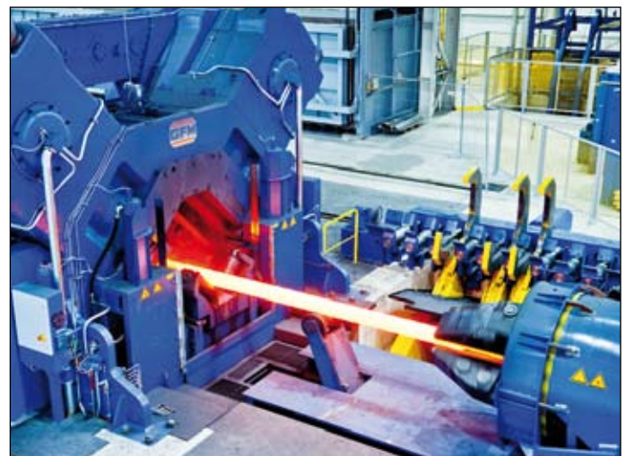
The plant is now capable of producing steel bars up to 15 metres long, with a diameter of up to 550 mm.
