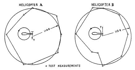
Area of discomfort due to a Hovering Helicopter Limit of discomfort — 10 knots
