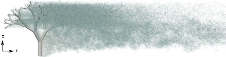
Figure 10. Isosurfaces of the second invariant of the velocity gradient tensor of the flow around Basic n = 8 at Re_H = 2500 and Re_H = 120000 . The wake region's opacity is adjusted to improve the visibility of the tree's branching part.
