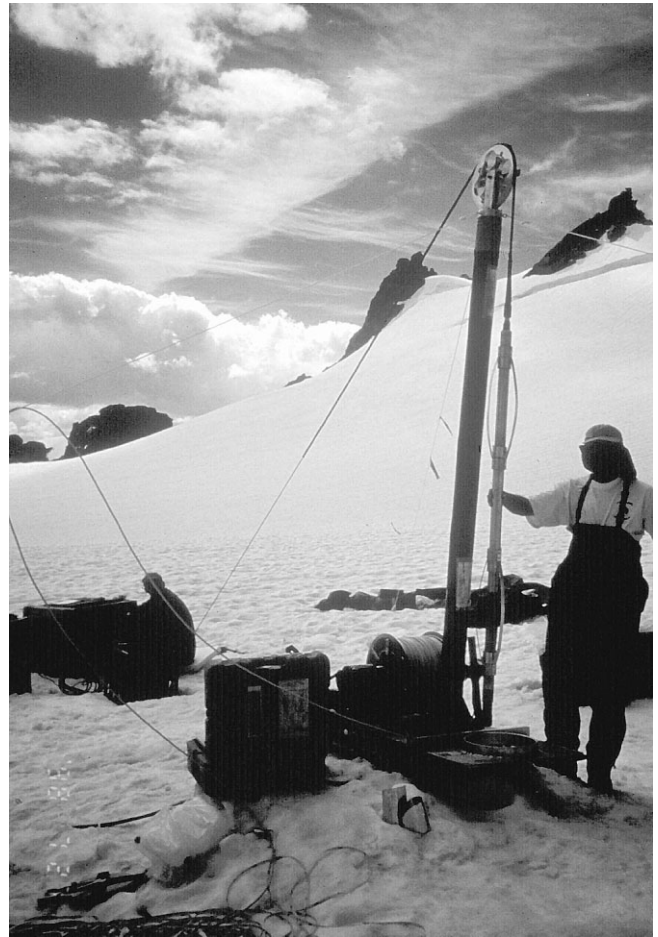
Fig. 2. Photograph of acoustic televiewer system deployed at study site, showing tool, cable, electric winch and thermal drill.
