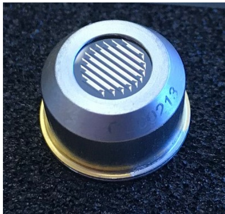
Figure 1. Vacuum encapsulated module with 150 nm graphenic window on a Silicon support grid
