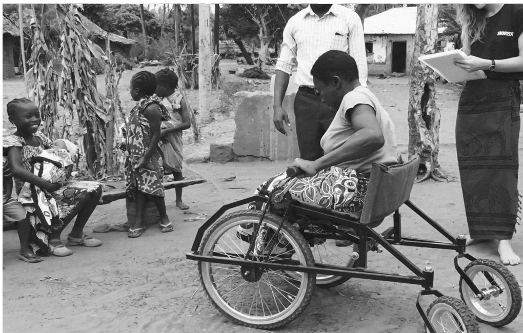
Figure 3. User's family watches as they test a new hand pedal wheelchair prototype.
