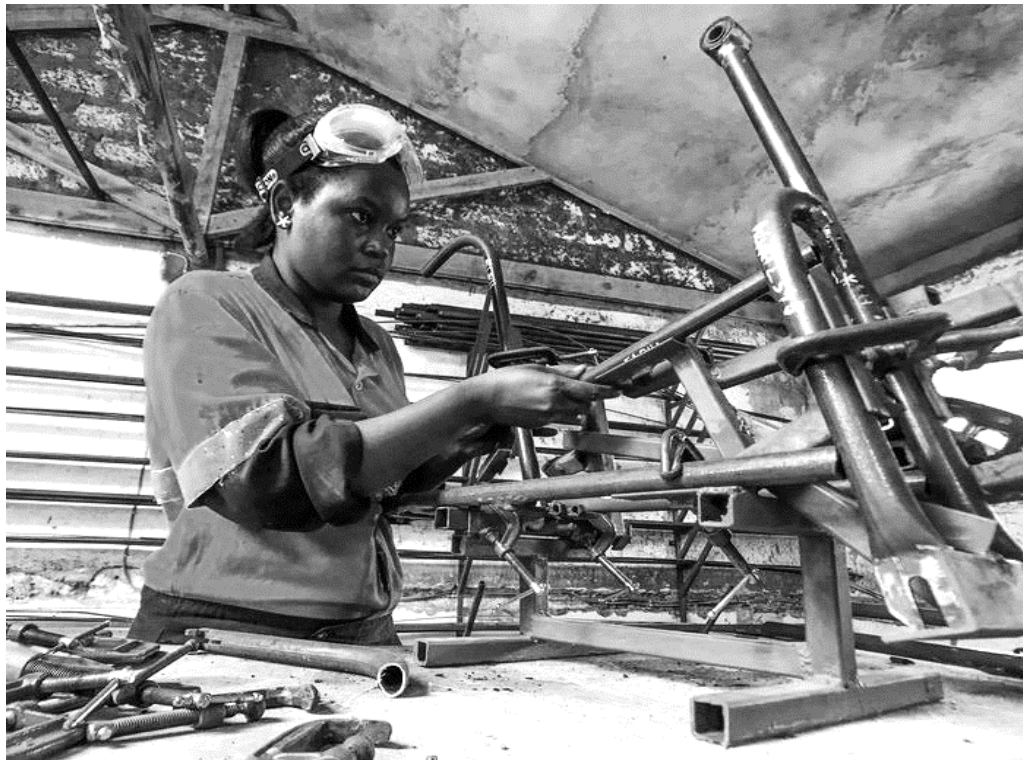
Figure 7. Using a jig to accurately position frame components in preparation for welding.
