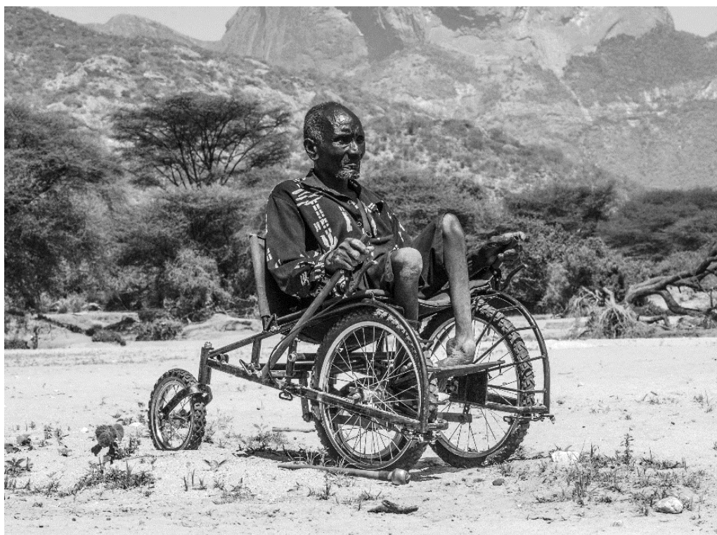
Figure 2. User testing the first lever-propelled wheelchair prototype with an articulated chassis acting as a suspension mechanism over uneven terrain.
