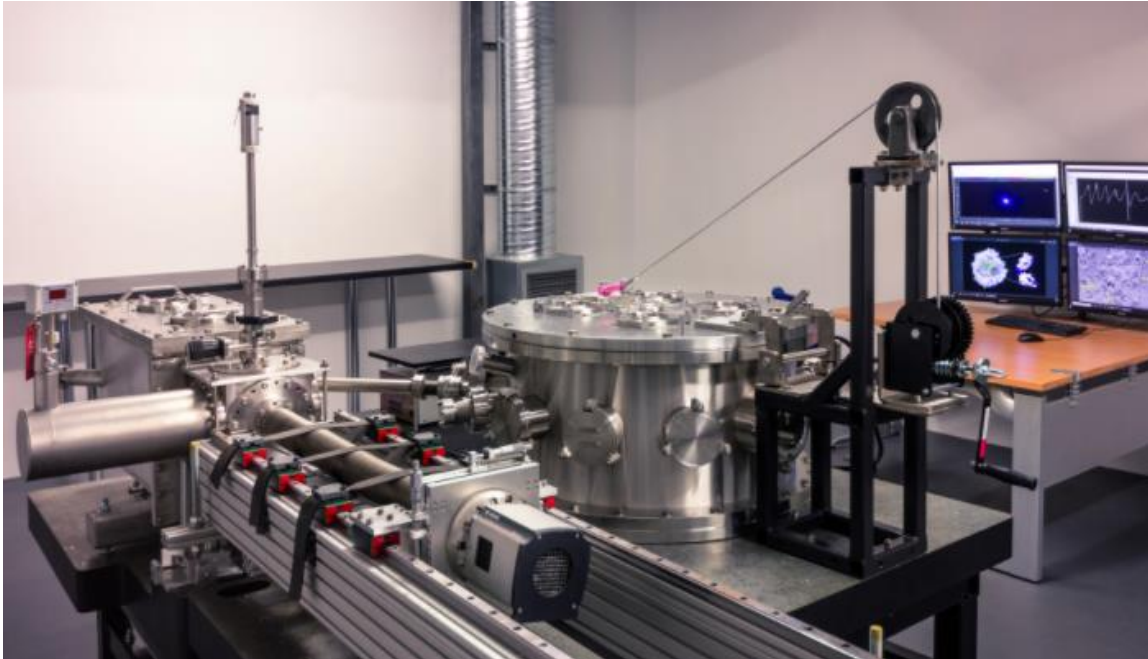
Figure 1. The SiriusXT Laboratory Scale Soft X-ray Microscope
