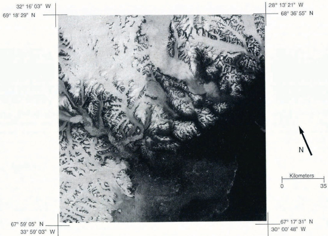
Fig. 2. First principal-component image computed from bands 1–4 of the 2 September 1988 Landsat TM data (scene-id YE22901288246, WRS-2 path 229, row 12).
