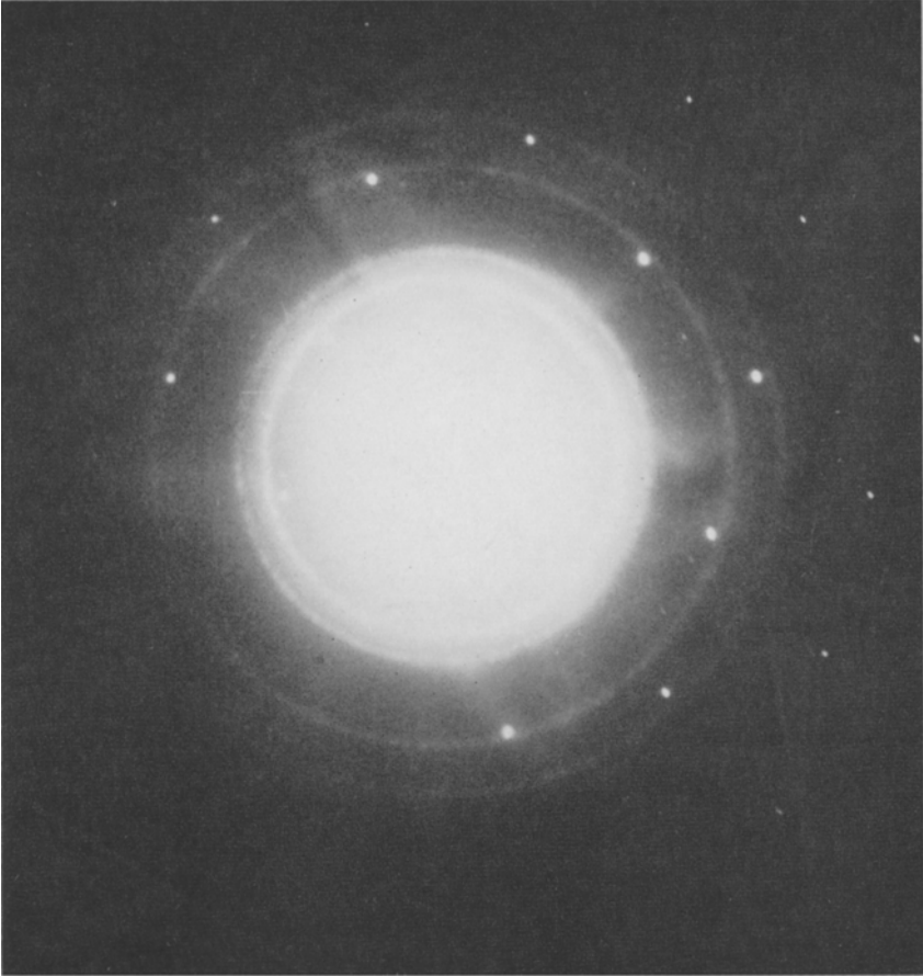
PLATE 3.—Electron diffraction pattern of cristobalite from talc heated at 1200°C.
