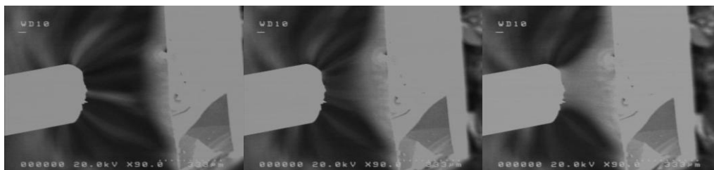
FIG. 3. Visualization of the water vapor flow from the nozzle as the nozzle-sample gap was reduced, from left to right image.
