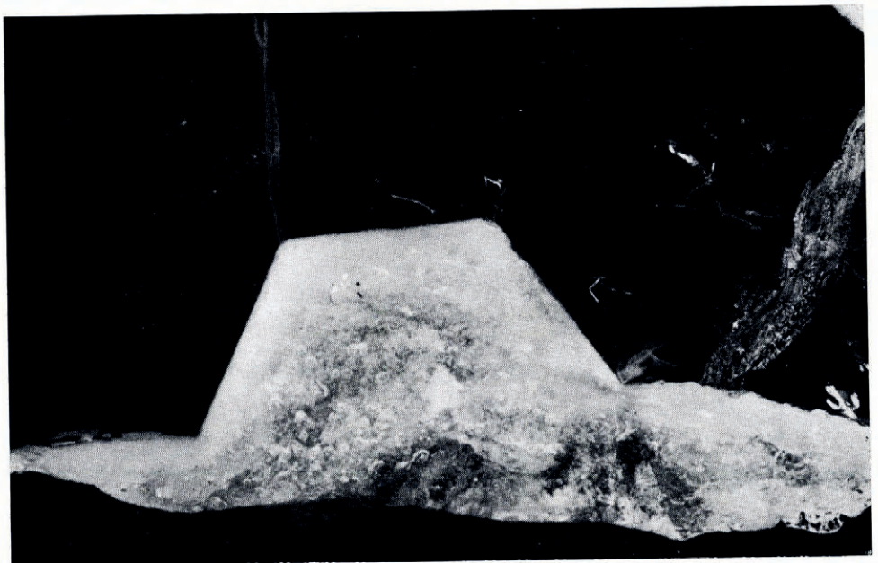
Fig. 9(a). An ice sample before regelation. A thin section cut from a sample grown around a hexagonal cylinder. The ice is lying on a black background.
