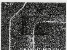
A contamination deposit was formed by a short SEM scan on a dirty specimen.
