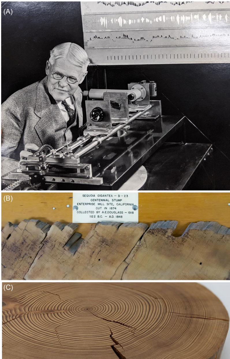
Figure 1 Early tree-ring and radiocarbon interactions: (A) Andrew Ellicott Douglass with his Cycloscope (1935), designed with the over-riding aim of discovering predictable cycles of solar activity in patterns of tree-ring growth, with emphasis on the 11-year solar cycle and its impact on climate (see Webb 1993 for further details). (B) Centennial Stump from California's Sierra Nevada used by Willard Libby in the first radiocarbon calibration, the "Curve of Knowns" featured in his Nobel prize speech in 1960. Note the large notches along the top edge of the sample created by the radiocarbon sampling. (C) Sample from "Broken Flute Cave," an Ancestral Puebloan cliff dwelling in the Prayer Rock district of the Navajo Nation in Arizona, also used in Libby's Curve of Knowns. (All images reproduced with permission from The Laboratory of Tree-Ring Research, University of Arizona.)
