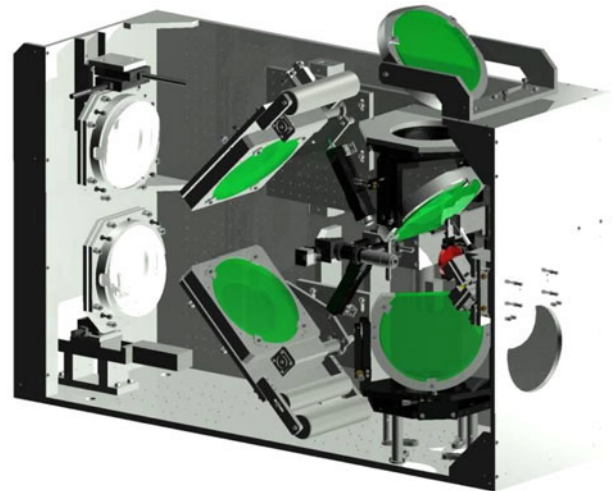
Figure 18. Double plasma mirror system on Astra-Gemini.
