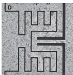
**Figure 1. Schematic device cross-section (A) and time series of BF STEM images of GST undergoing phase change (B-D).** The device consists of an electron transparent Si<sub>3</sub>N<sub>4</sub> membrane, a Pt heater, a layer of ALD Al<sub>2</sub>O<sub>3</sub>, a pair of Pt electrodes, and a thin film of GST. The GST is amorphous (B) as deposited. It changes from amorphous to fcc (C) to hexagonal (D) as the heater power is increased.
