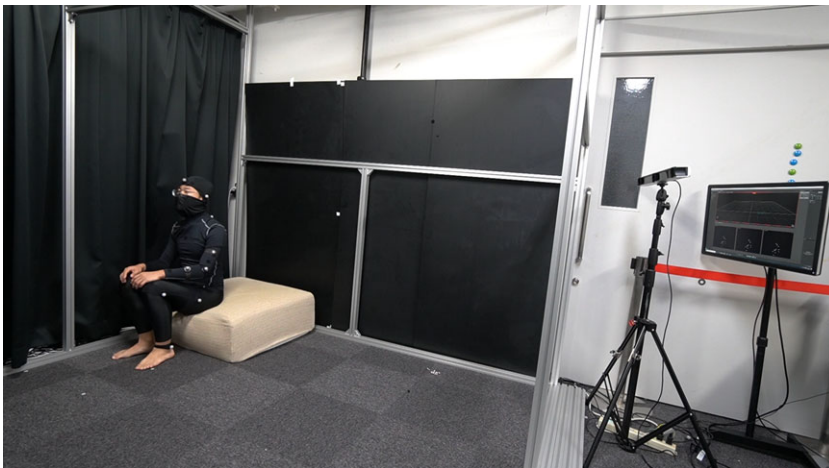
Figure 10. The configuration of the motion capture system and the captured subjects. The OptiTrack motion capture system is used to detect the markers' locations in the set coordinate frame. Capture frame rate: 120fps, export frame rate: 120fps. Rotation type: quaternion.
