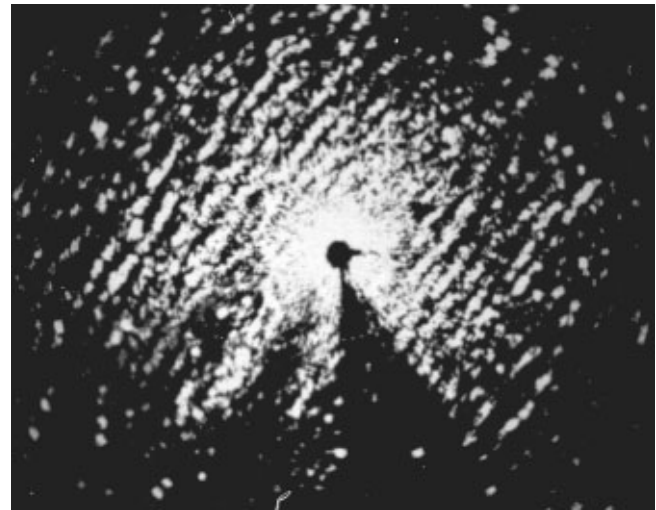
Fig. 1. The ship's radar screen at the time of the measurements. North is upwards. Wave crests due to waves from bearing 305° are visible.
