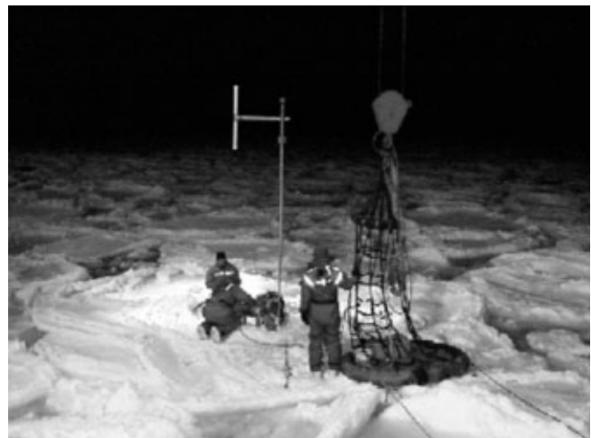
Fig. 2. Deploying the instrumentation on an ice floe from a basket lowered over the side of the ship.
