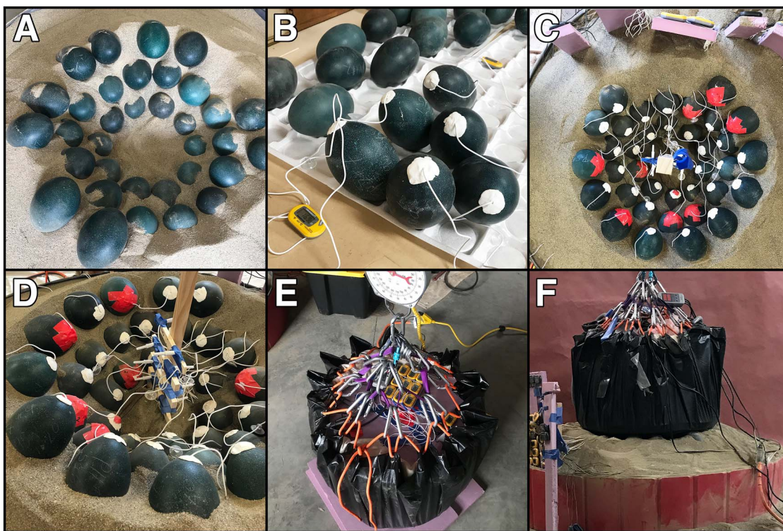
Figure 3. Photographs of the experimental arrangement. A, Nonviable emu eggs placed in a three-level oviraptorosaur-style clutch before experimentation. B, The blunt end of each egg was carefully tapped open to allow a thermometer to be placed inside before resealing. C, Eggs back into place with thermometers inserted. D, Close-up of experimental eggs. Central column probes are visible attached to a stake in the middle of the clutch (stake top was truncated before tests were run). E, Surrogate dinosaur seen from above. It held ~70 kg of water, heated to approximately 39°C, and had a total mass of ~80 kg. F, Surrogate shown as it looked while resting on the nest in all experiments.
