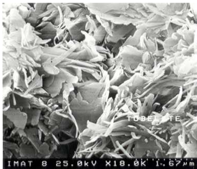
Fig. 7. Scanning electron microscopy of \text{NH}_4\text{-I} crystals exhibiting a platy- and lath-shaped morphology.
